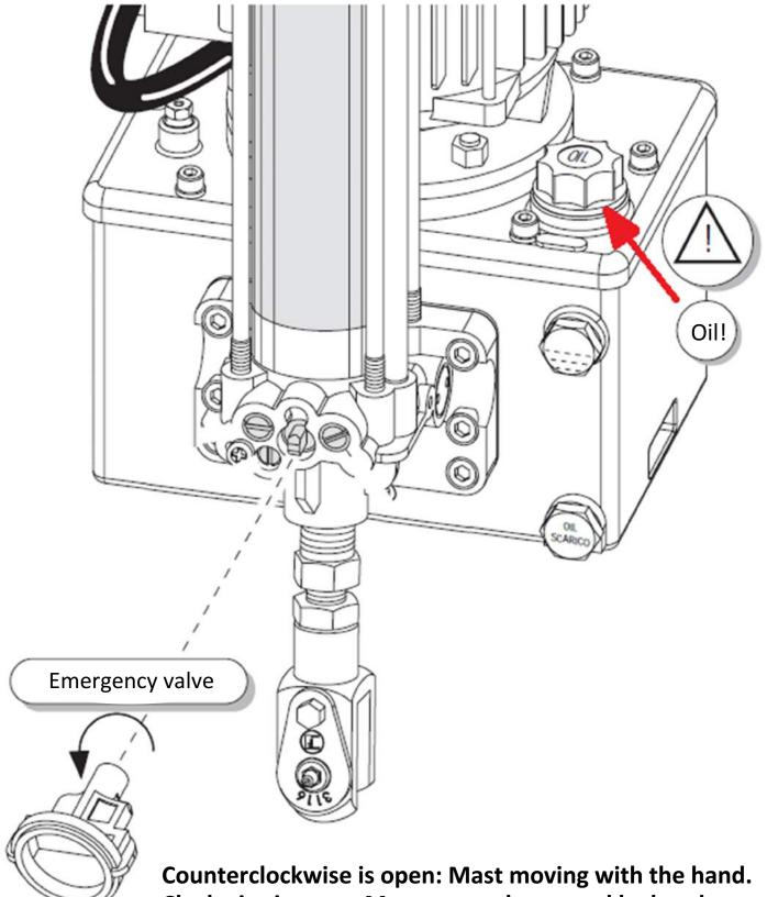
Clockwise is open: Mast cannot be moved by hand.
